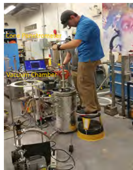
Experiments at NASA-SWAMPWORKS using UCF asteroid regolith simulant. This was to determine the strength of an icy regolith.
