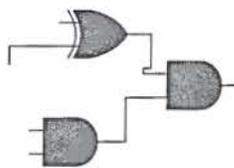
**Combinatorial Logic:** Output is a function of the inputs after some delay ( $\tau_{dly}$ )
