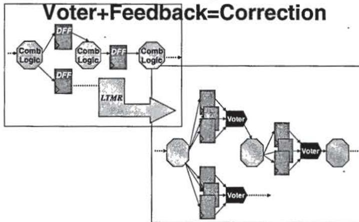
$$P(f_s)_{error} \propto P_{configuration} + \underbrace{P(f_s)_{functionalLogic}}_0 + P_{SEFI}$$
