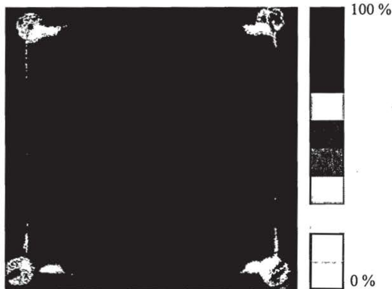
Figure 13. C-scan of melt mixed 0.5 wt % MWCNT/PETI-330/M55J PMC.
