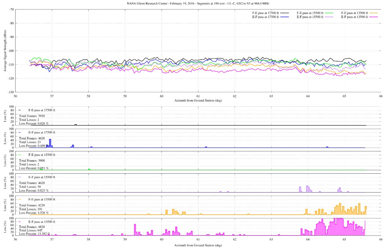
Figure 28.—Uplink L-band signal strength and frame loss versus bearing angle over hilly terrain at 35-nmi range.
