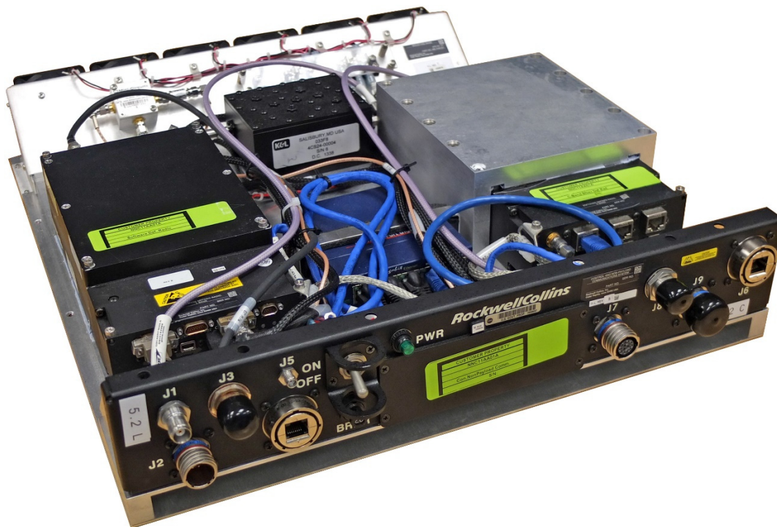
Figure 1.—Control and Non-Payload Communications (CNPC) radio tray including L-band radio (left) and C-band radio (right) with attendant cabling and interface components.
