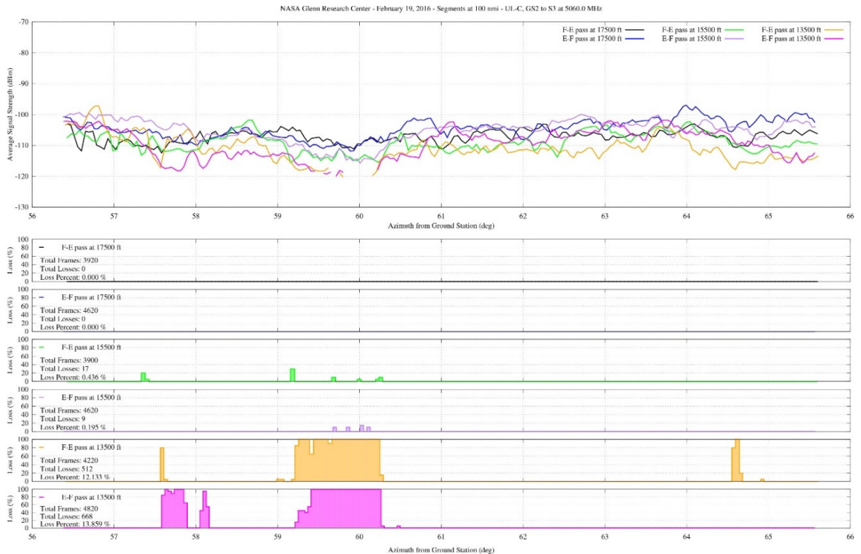
Figure 25.—Uplink C-band signal strength and frame loss versus bearing angle over hilly terrain at 100-nmi range.
