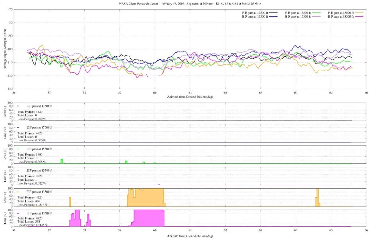
Figure 24.—Downlink C-band signal strength and frame loss versus bearing angle over hilly terrain at 100-nmi range.
