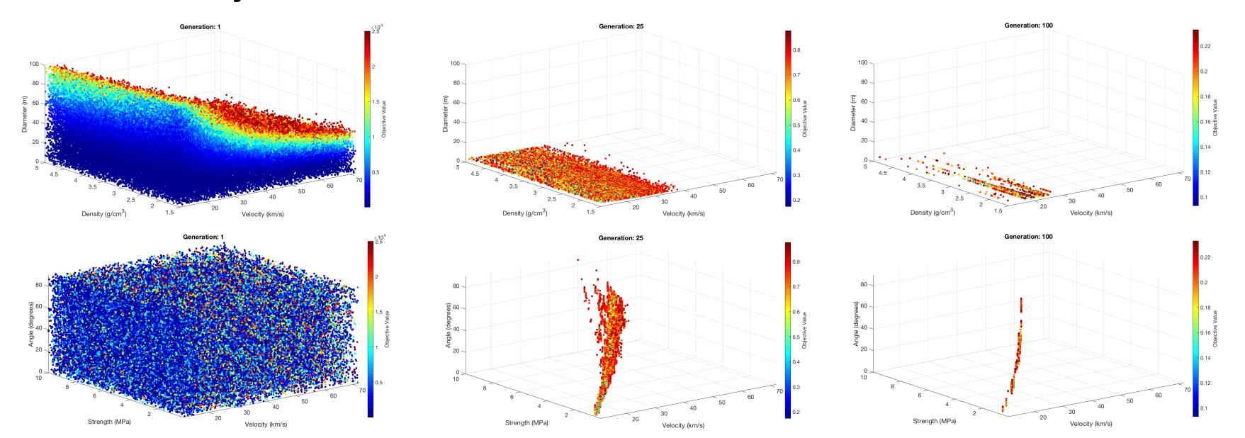
The GA reveals the error space and how genes evolve. The figures above demonstrate that diameter denotes a surface where only few solutions are possible. This well demarcated surface is contrasted by the scatter plot of strength, angle, and velocity, where there is no recognizable surface.
