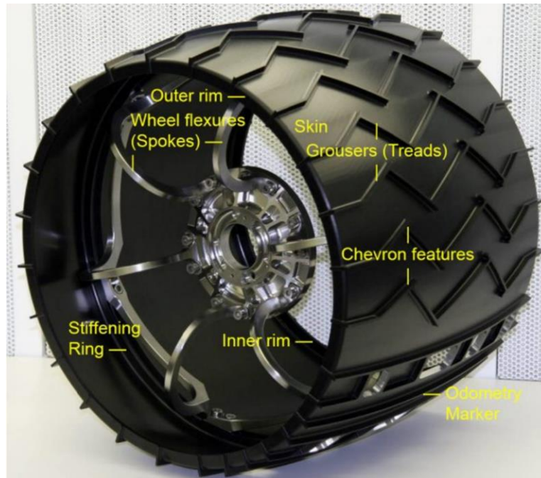
Figure 3. Curiosity's wheel made from a single piece of machined aluminum alloy AA7075-T7351. The main rim is 1.9 cm thick (0.75-inches).
