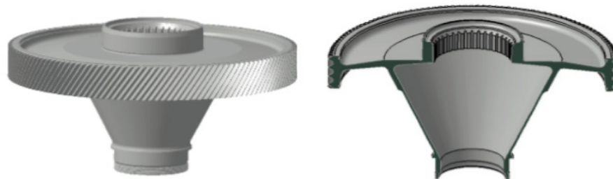
Figure 3.—Bull Gear Candidate
