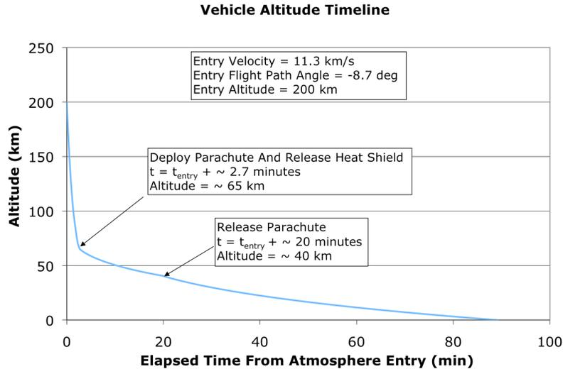
Figure 5.8—Nominal altitude profile during atmospheric entry.
