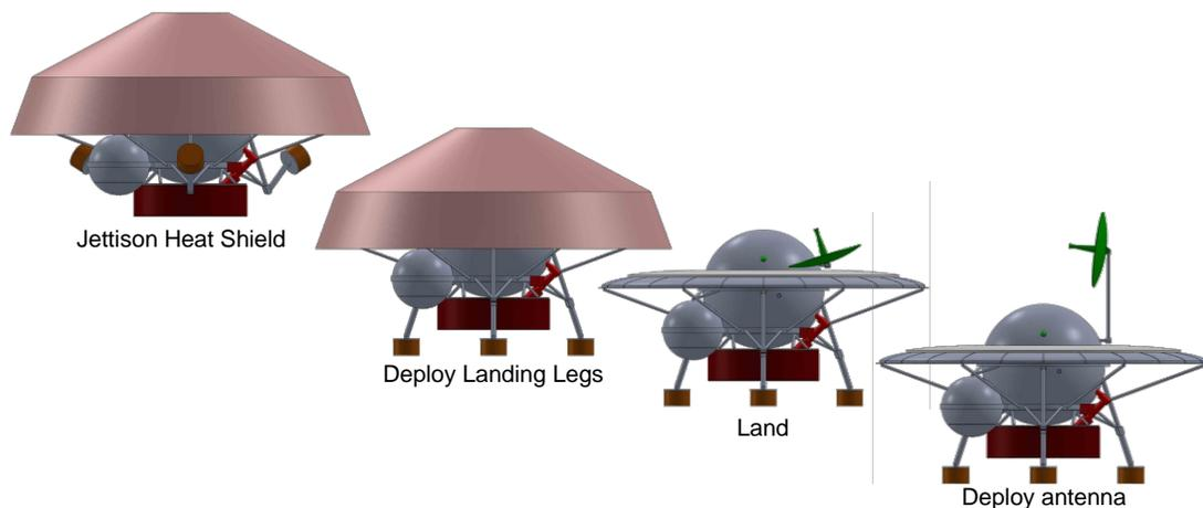
Figure 2.19—Landing legs and X-band antenna deployment sequence.
