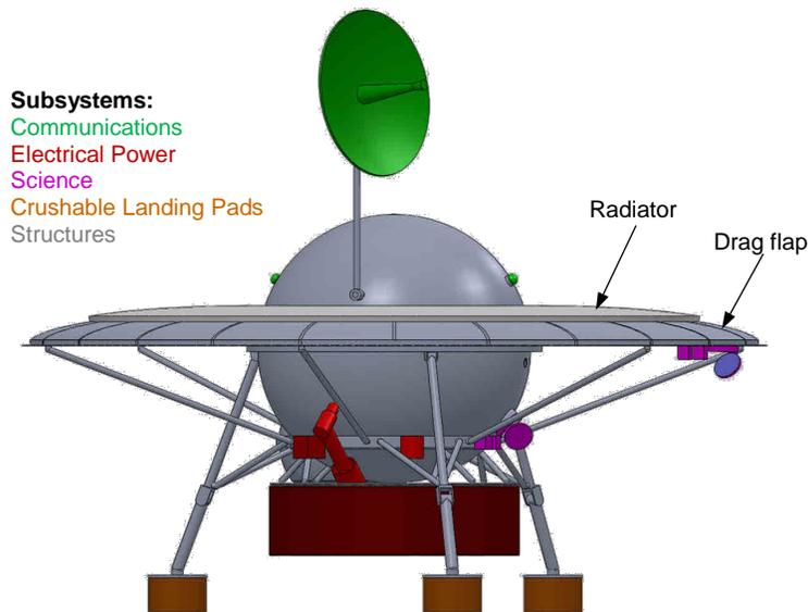
Figure 3.1—ALIVE design approach—External components.
