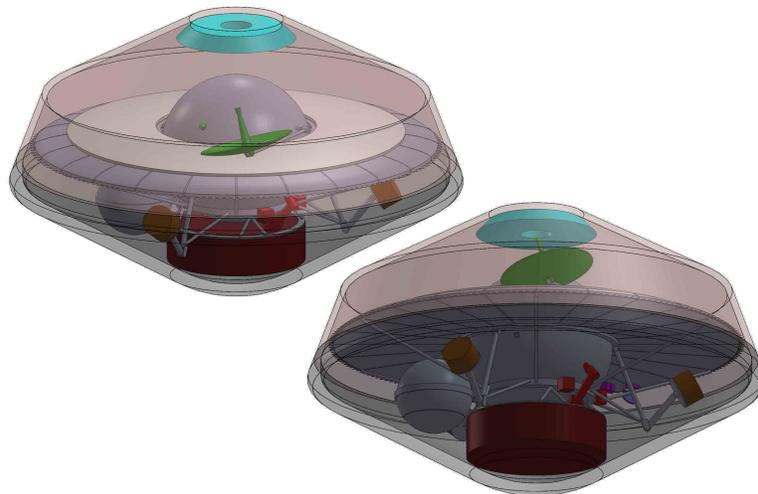
Figure 2.18—Isometric views of the ALIVE Lander inside the aeroshell.
