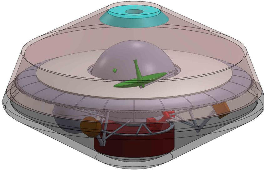
Figure C.1—ALIVE stowed configuration for interplanetary flight
