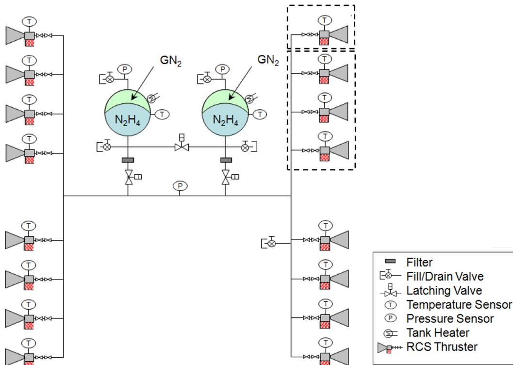
Figure 5.13—Preliminary Cruise Deck Propulsion P&ID.
