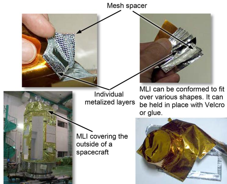
Figure 5.16—Example of MLI blanket design and application.
