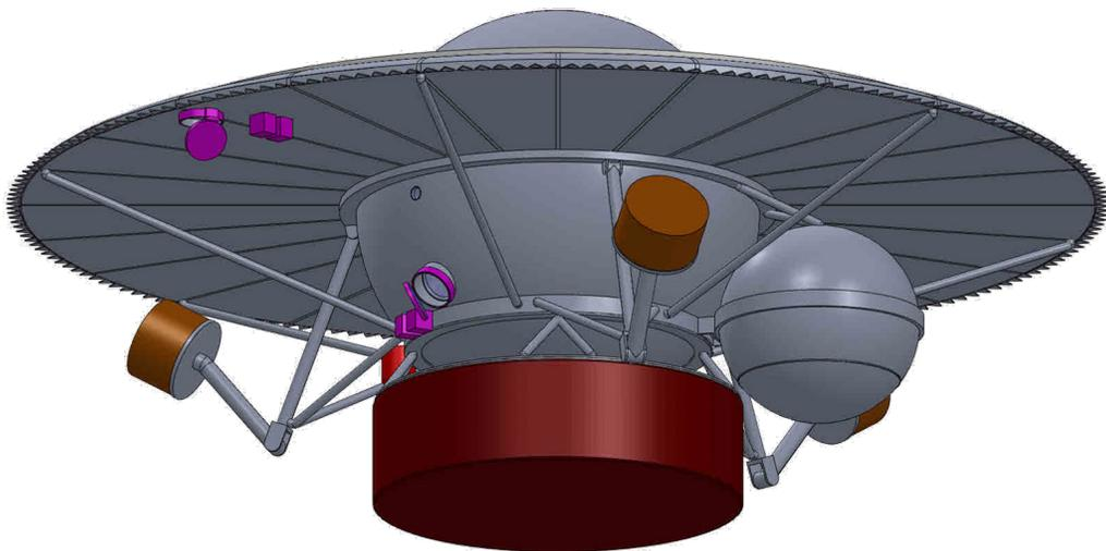
Figure C.2—ALIVE after jettison heat shield while deploying for landing
