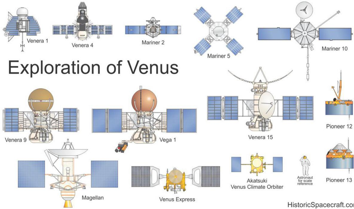
Figure 2.1—Previous Venus space vehicles. (Used with permission from Richard Kruse. Image can be found at [http://historicspacecraft.com/Diagrams/P/Venus\\_Probes\\_RK2014\\_1200x700.jpg](http://historicspacecraft.com/Diagrams/P/Venus_Probes_RK2014_1200x700.jpg)).
