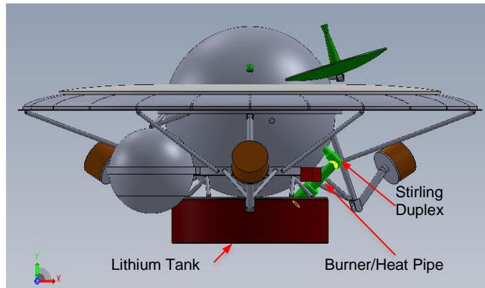
Figure 5.12—ALIVE Power/Cooling System highlights.
