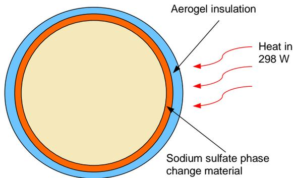
Figure 5.21—Descent electronics thermal control items.
