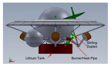
Figure 5.12—ALIVE Power/Cooling System highlights.
