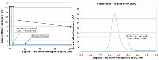
Figure 5.7—Acceleration timeline from atmospheric entry.
