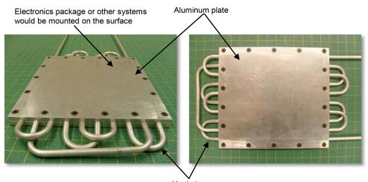
Heat pipes Figure 5.17—Example of a cold plate with integrated heat pipes.
