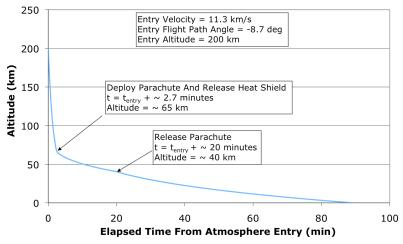
Figure 5.8—Nominal altitude profile during atmospheric entry.
