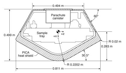
Figure 5.20—Stardust Aeroshell geometry.
