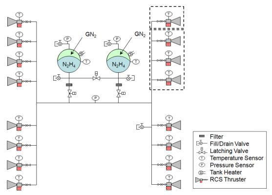
Figure 5.13—Preliminary Cruse Deck Propulsion P&ID.
