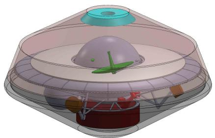
Figure C.1—ALIVE stowed configuration for interplanetary flight
