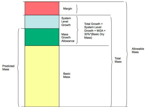
(Basic = bottoms-up estimate of dry mass. Mass growth allowances (MGA) = applied per subsystem line item) Figure 2.4—Graphical illustration of the definition of basic, predicted, total and allowable mass.
