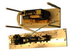
Figure 5.5—Image of representative TWTA and Electronic Power Conditioners (EPC).
