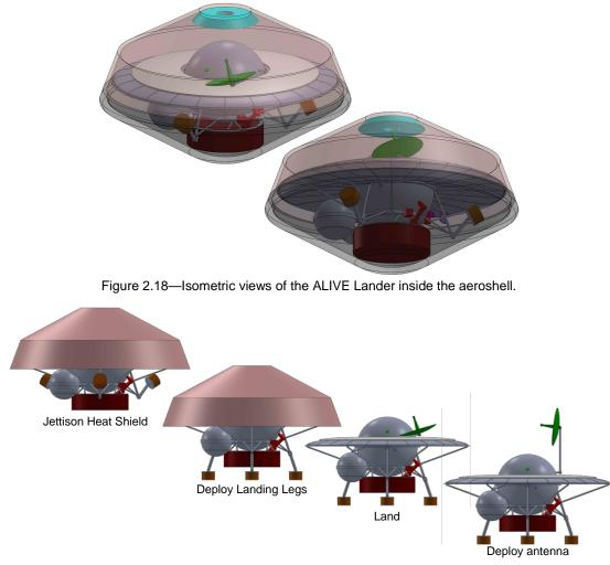
Figure 2.19—Landing legs and X-band antenna deployment sequence.
