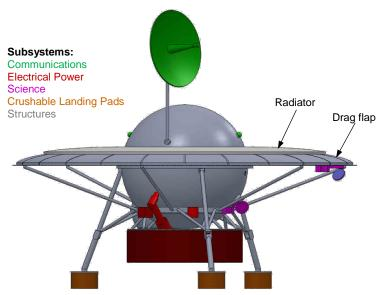
Figure 3.1—ALIVE design approach—External components.
