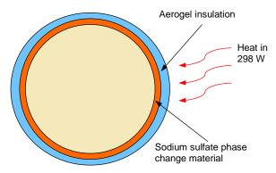
Figure 5.21—Descent electronics thermal control items.
