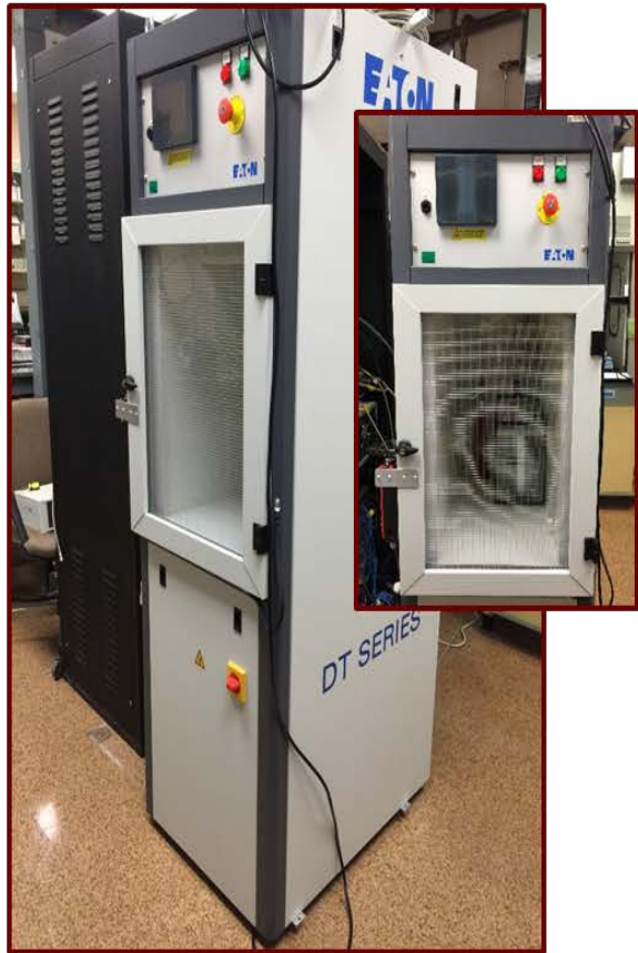
Eaton High Voltage Test Set Located at NASA GRC 106:B10
