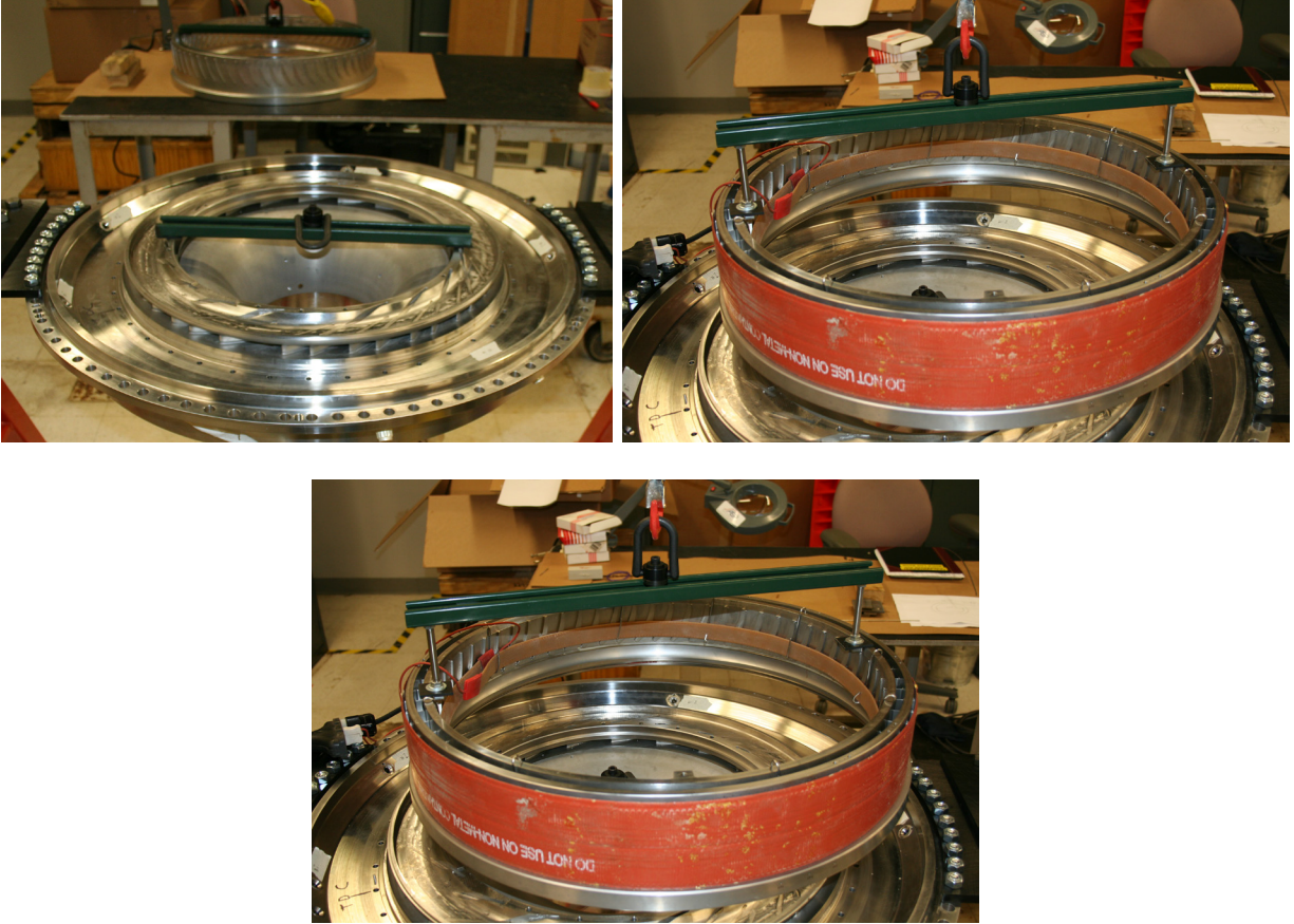
Figure 94.—Steps involved in the mock assembly. First (top left) placement of the diffuser subassembly on the shroud. Then placing the heat belts around the EGV surfaces and heating it to about 150~160 °F. At that time EGV subassembly is lifted with a crane and moved over the shroud (top right), and lowered using a locating pin. Finally, the removal of the heating pads and check for the fit (bottom picture).
