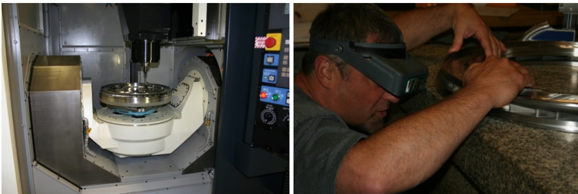
Figure 92.—Diffuser assembly being inspected at UTRC on the 5-axis machine (left), as well as visually.
