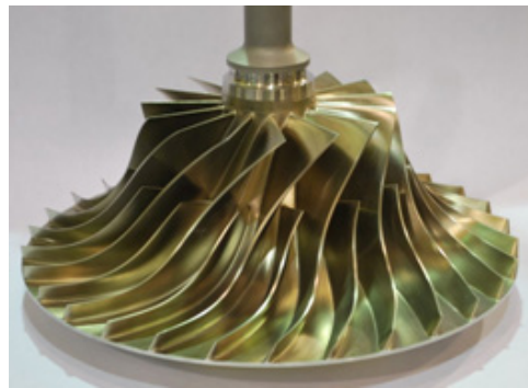
Figure 79.—HECC impeller after the final machining.
