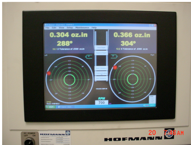
Figure 84.—The Hoffmann machine showing the imbalance readings after regrinding of the curvic couplings and the impeller. These readings are 10 times larger than the imbalance specified on the drawings.
