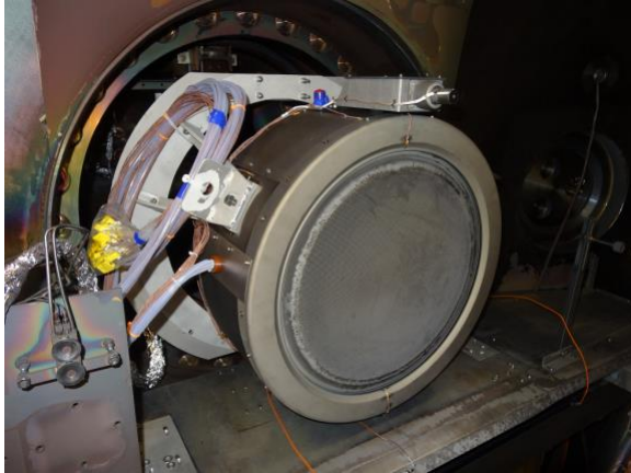
Fig. 2: NEXT-C Dev-C thruster.
