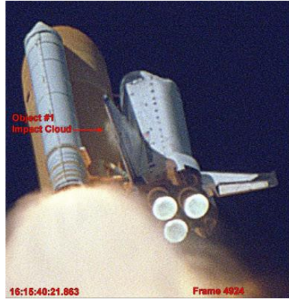
Crew of the Space Shuttle Columbia (left): (l. to r.) Mark Brown, Rick Husband, Laurel Clark, Kalpana Chawla, Mike Anderson, Willie McCool, and Ilan Ramon. Foam debris at moment of impact during launch of Columbia (right). Images courtesy of NASA.
