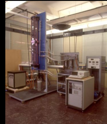
Falling-Film Heating/Evaporation Facility
