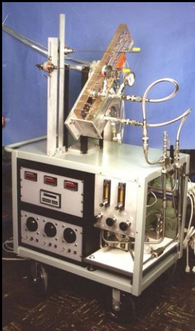
One-G Flow Boiling Facility
