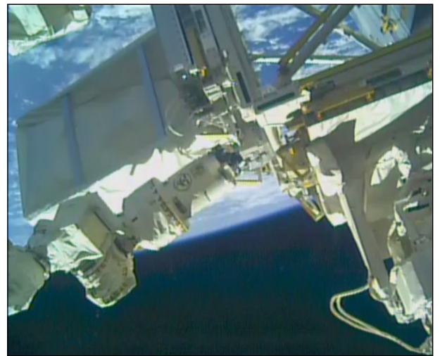
Figure 4. SDS installed on the EPF-SOX platform; SPDM OTCM preparing to detach and walk away.
