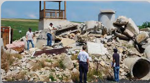
Researchers performing a test of the FINDER prototype. The device uses radar technology to sense the heartbeats and breathing of humans hidden behind piles of rubble.
