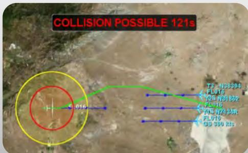
NASA developed a system (collision-avoidance algorithm, sophisticated display options) to meet/exceed FAA requirements for UAS.
