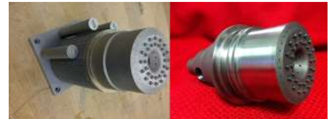
One-piece as-built (left) and post-processed (right) rocket engine injector made in 40 hours at NASA MSFC
