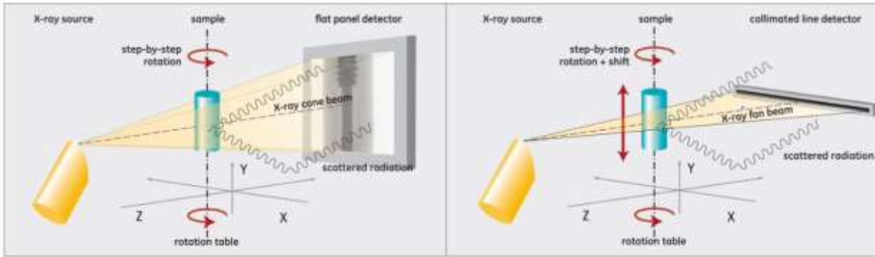
Cone beam CT (3D) is fast but scattered radiation can affect the image quality
