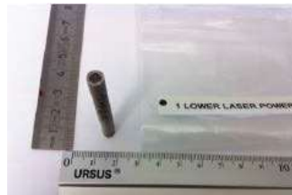
Concept Laser Inconel 718 prisms for CT capability demonstration
