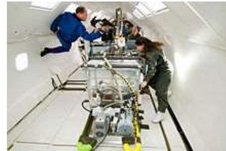
EBF 3 wire-fed system during parabolic flight testing
