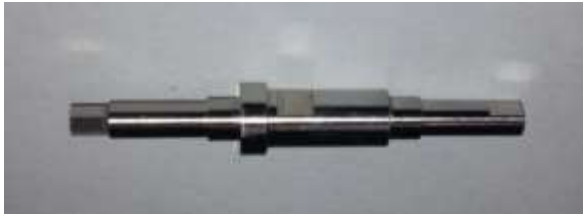
JPL Mars Science Laboratory Cold Encoder Shaft fabricated by gradient additive processes
