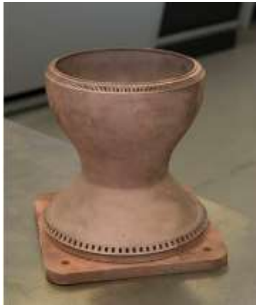
MSFC copper combustion chamber liner for extreme temperature and pressure applications
