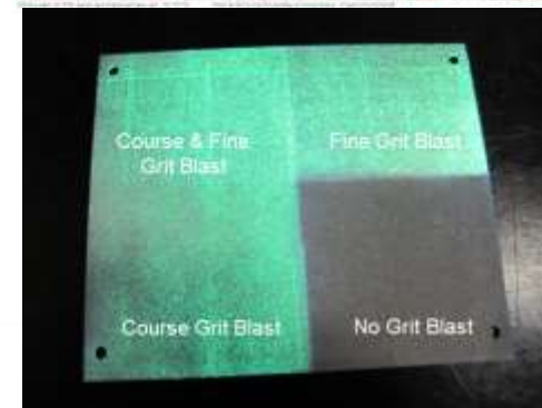
Effect of sand grit blasting on PT results: visible images (top), 200x micrographs (middle), and UV images of grit-blasted surfaces with penetrant applied (bottom)
