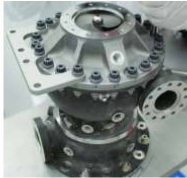
MSFC rocket engine fuel turbopump with 45 percent fewer parts than pumps made with traditional manufacturing
