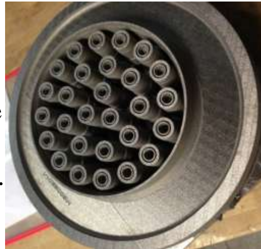
28-element Inconel ® 625 fuel injector built using an laser powder bed fusion (L-PBF) process
