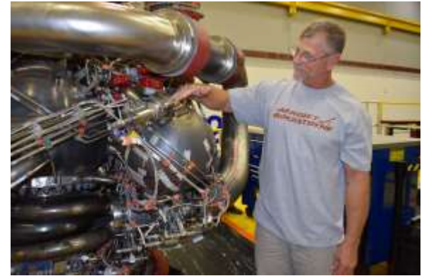
A technician for NASA's RS-25 prime contractor Aerojet Rocketdyne exhibits the pogo accumulator assembly, NASA's largest 3D-printed rocket engine component tested in the restart of RS-25 production.
