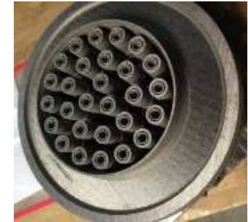
28-element Inconel 625 fuel injector
