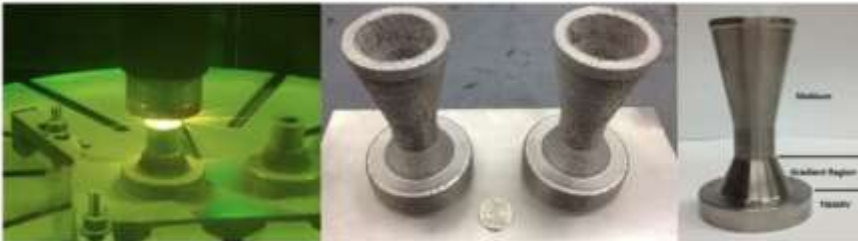
Prototype titanium to niobium gradient rocket nozzle
