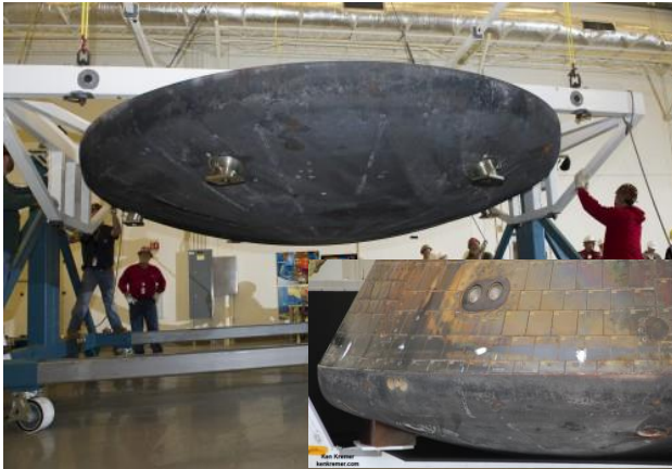
Figure 7 EFT-1 Heat Shield in Post Flight Evaluation
