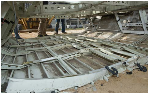
(a) Bottom centerline failures.
