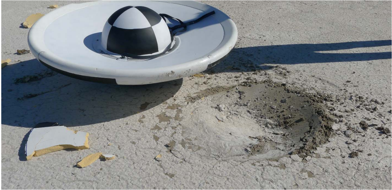
Figure 26 - Test 3 impact location and crater
