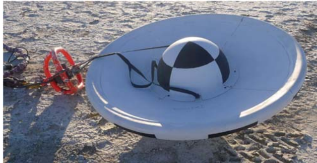
Figure 4 - Test vehicle shown with release hook (in orange) attached to vehicle's three point harness.
