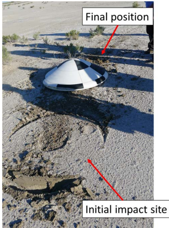
Figure 21 - Test 2 impact location and crater
