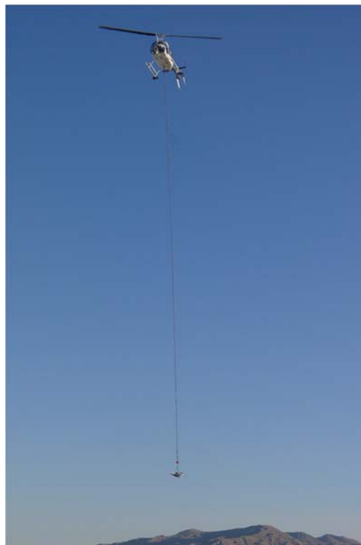
Figure 5 - Test vehicle attached to helicopter via a 33 m long lanyard
