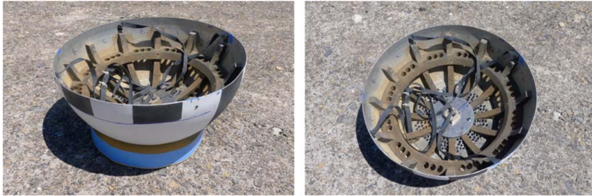
Figure 6 - Drop penetrometer used for practice testing. Side view on cradle (left) and top view (right)
