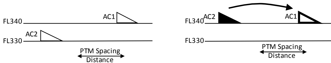
Figure A.6 PTM operations during altitude change maneuvers.
