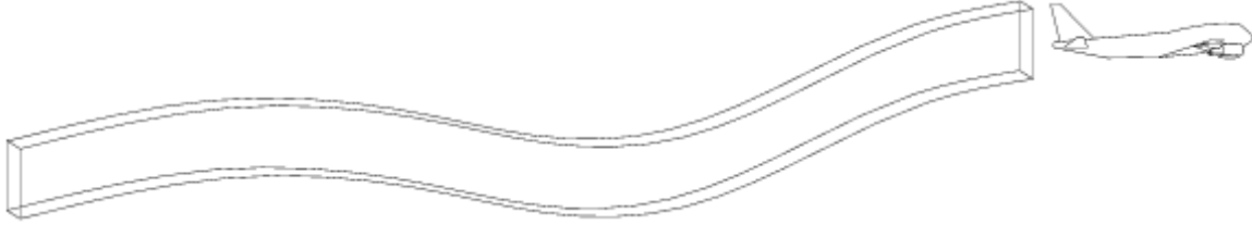
Figure 3-1. Wake vortex containment region.
