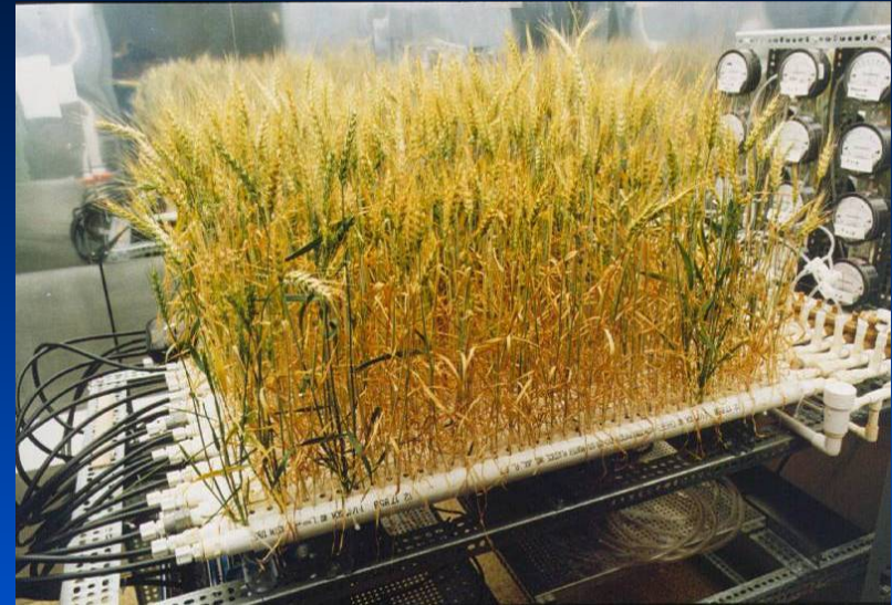
Porous Ceramic Tubes to Contain the Water
