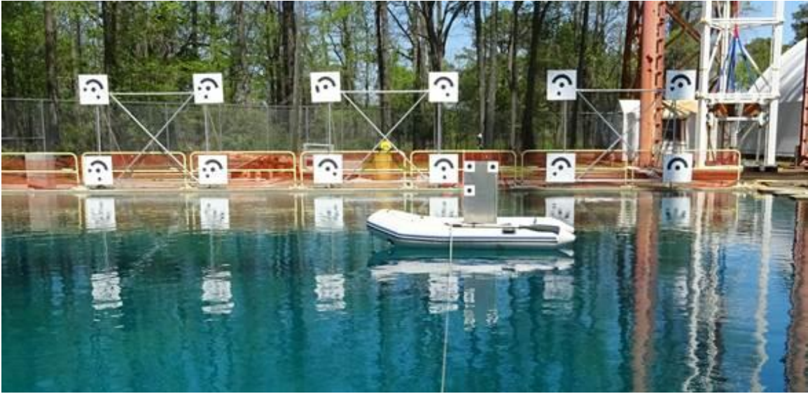
Figure 18. Photogrammetry Coordinate System Targets
