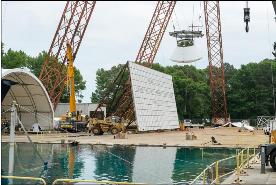
Figure 5. Test Set-up for a Representative GTA WIT Swing Test with Horizontal Velocity
