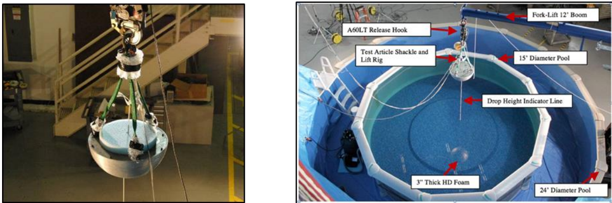
Figure 1. EWIT Phase 1 Test Article and Test Set-up
