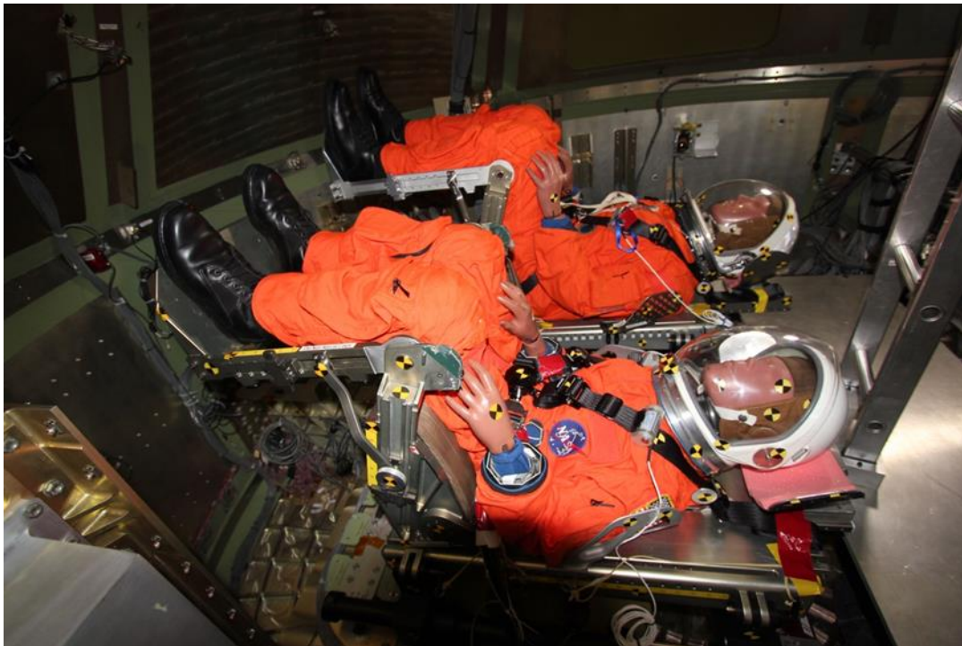
Figure 4. Anthropomorphic Test Devices Installed in the GTA
