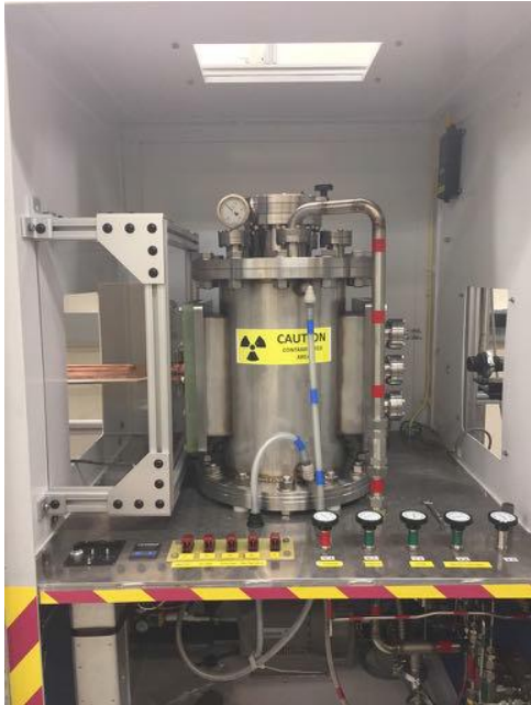
Figure 19: Compact Fuel Element Environmental Test system
