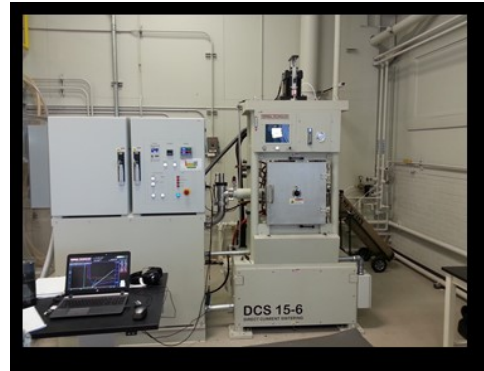
Figure 12: Direct Current Sintering Machine at Marshall Space Flight Center
