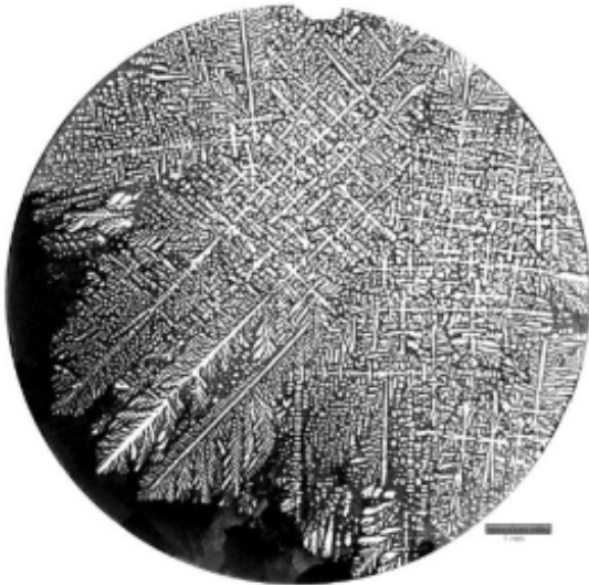
Pb-Sb Anisotropic dendrite formation
