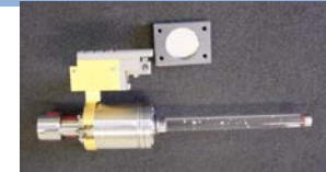
DSI-R Cartridge during preparation including Succinonitrile-camphor sample material
