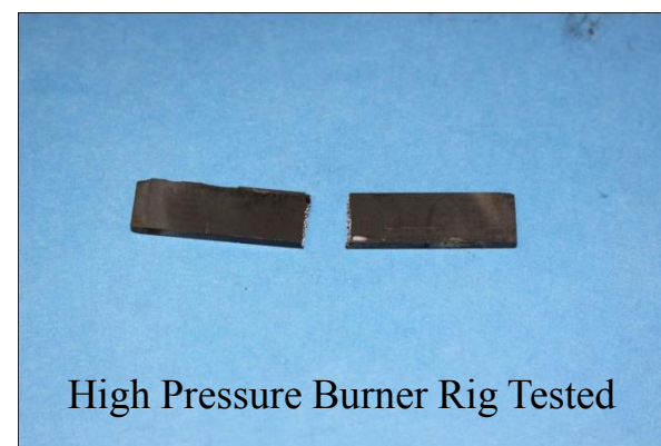
Examples of Tyrannohex composites failure after testing
