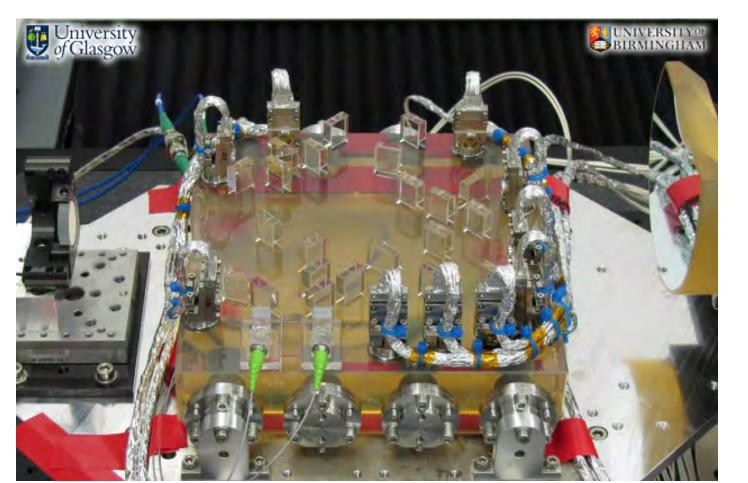
**Using hydroxy-catalysis bonding** techniques, we can build complex optical structures with picometer-level dimensional stability and high mechanical strength. The optical bench [1] for LISA Pathfinder enabled stable precision laser interferometry that enabled the spectacular results show below. The LISA optical bench will use the same construction methods, and they may be applied to other instruments (see below) and missions that require large stable telescopes.
