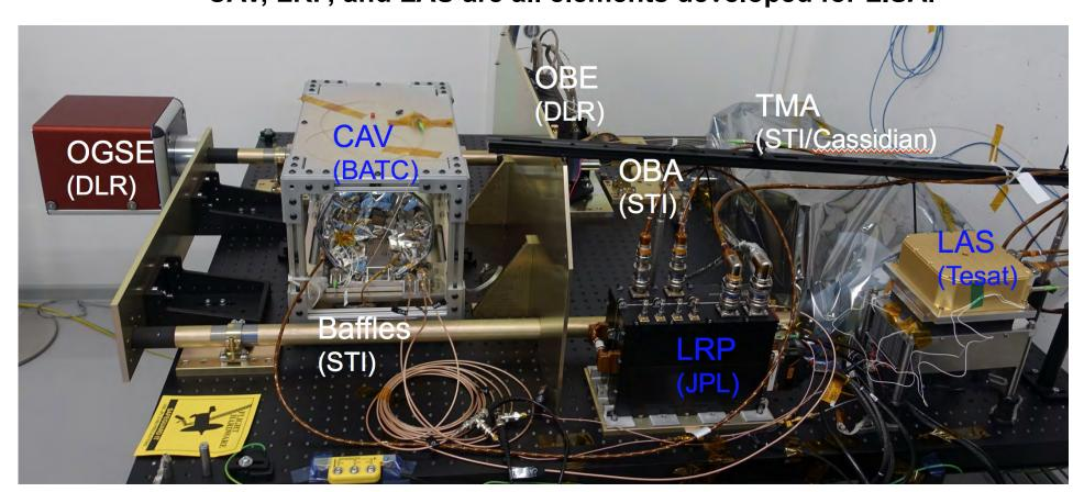
**Measured Frequency Stabilization Exceeds both LISA and GRACE FO requirements** Elements of the technology originally
