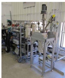
Soil Processing Module 10kg per batch; 5 kg/hr 0.15 kg/hr H 2 O (3% water by mass)
