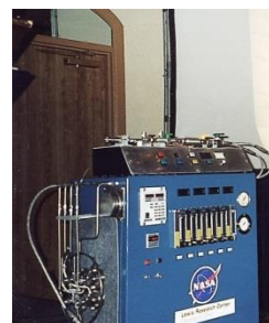
CO 2 Electrolysis (GRC) [Tested under conference conditions]
