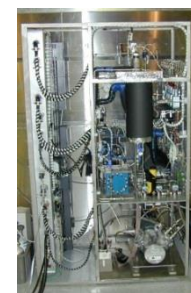
CO 2 Electrolysis (GRC) [Tested under conference conditions]
