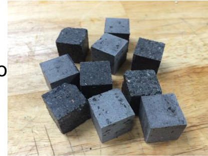
Standard 2-inch cube compression test specimens
