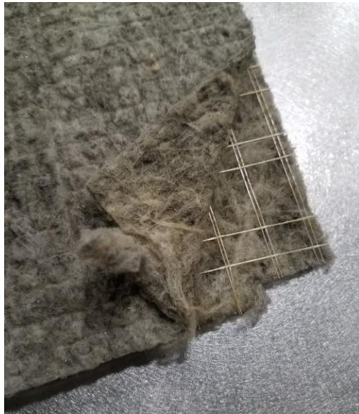
FIGURE 10: UAI FIBERGLASS INSULATION WITH EMBEDDED INTUMESCENT GRAPHITE FLAKES AND SCRIM.
