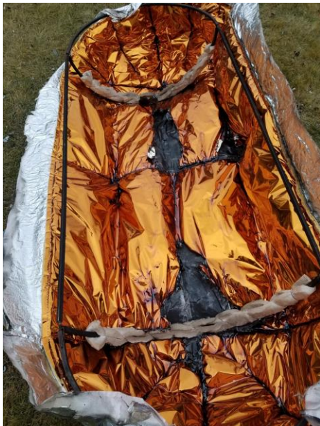
FIGURE 23: TYPICAL DOUBLE SHELTER INTERIOR POST-TEST CONDITION.
