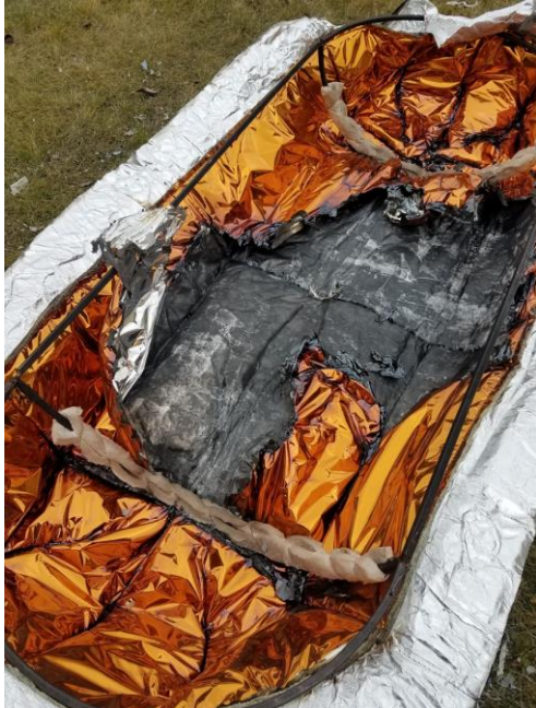
FIGURE 21: TYPICAL SINGLE INTERIOR POST-TEST CONDITION.
