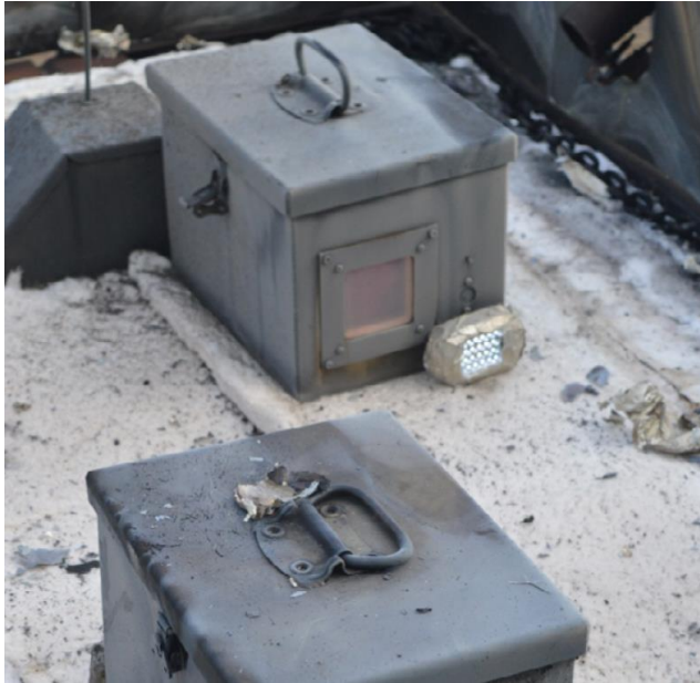
FIGURE 18: WHITE POWDER COVERING SHELTER INTERIOR INSTRUMENTATION AFTER THE CONCLUSION OF A SINGLE SILICONE SHELTER TEST.
