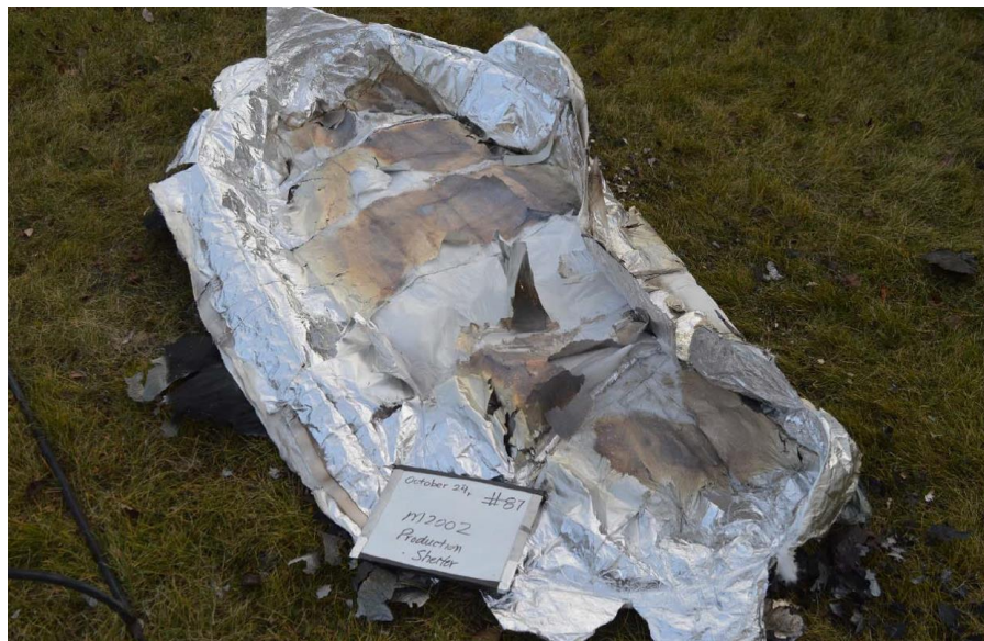
FIGURE 19: TYPICAL M2002 INTERIOR POST-TEST CONDITION.
