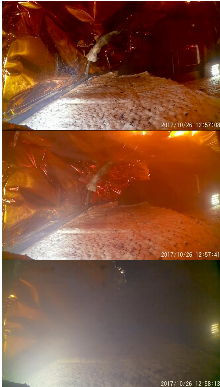
FIGURE 20: INTERIOR VIDEO DATA SHOWING SUBJECTIVE SMOKE CONCENTRATION INSIDE A SINGLE SILICONE SHELTER AT THREE TIMES: TEST CRITERION FAILURE (87 SECONDS, TOP), TEST CONCLUSION (119 SECONDS, MIDDLE), AND CONCLUSION OF VIDEO DATA (152 SECONDS, BOTTOM).
