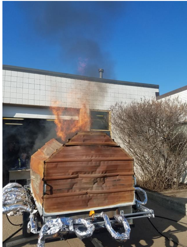
FIGURE 6: FULL SCALE SHELTER TEST APPARATUS AT THE UNIVERSITY OF ALBERTA WITH FLAMES ON DURING TESTS.
