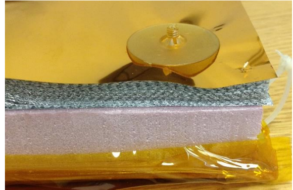
Figure 2. An MLI standoff holding the MLI blanket and foam insulation to the metal surface.
