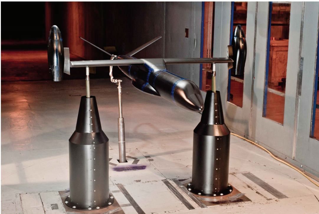
Figure 16: The L95 model configuration mounted inside the wind tunnel with round fairings.
