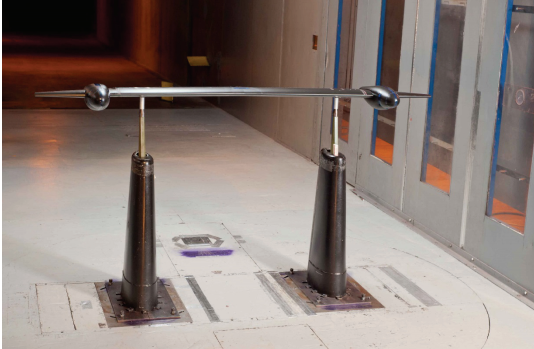
Figure 19: The WNE2L wing-only configuration mounted inside the wind tunnel with aerodynamic fairings.
