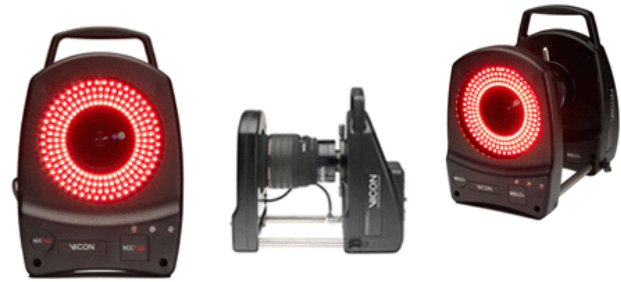
Figure 1. Vicon F40 camera showing ring LED lamp.
