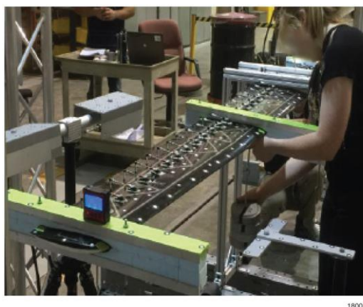
Figure 12. Photogrammetry testing of APV-3 wings.
