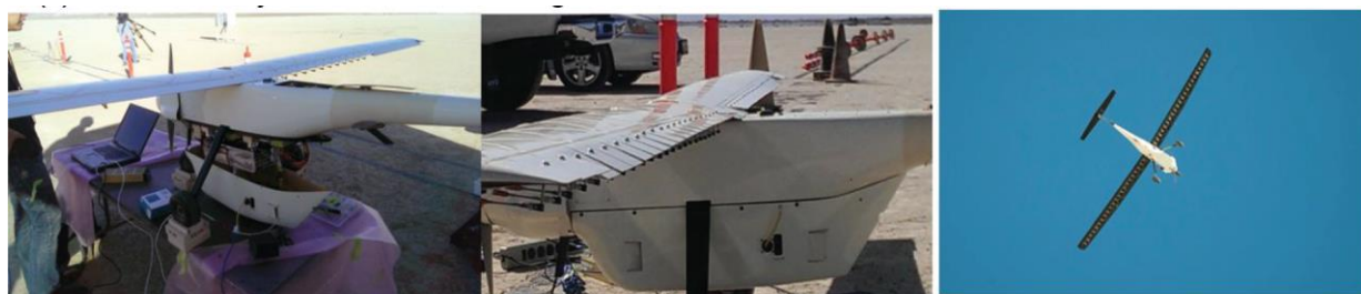
Figure 14. (a) Pre-flight checks of the cFOSS system and the SCS control system during one of the work-up flights, (b) complete systems ground test prior to flight, and (c) fully-modified APV-3 in flight.
