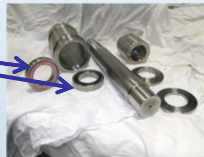
DA Centrifuge Bearing Test Rig Spindle Components
