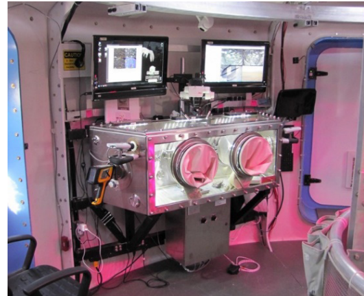
Fig. 1: GeoLab Glovebox integrated into the HDU during Desert RATS analog operations in 2010, 2011, and 2012.
