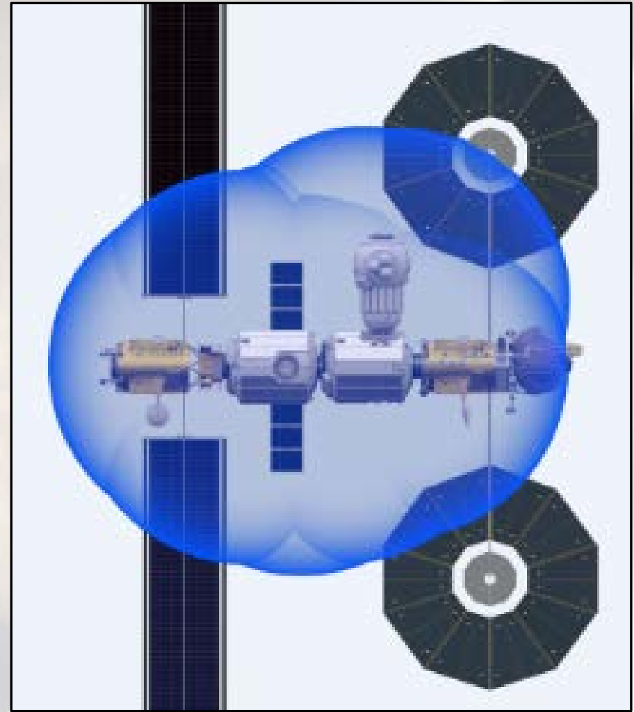
Robotically Assisted EVA with APFR Access Envelopes
