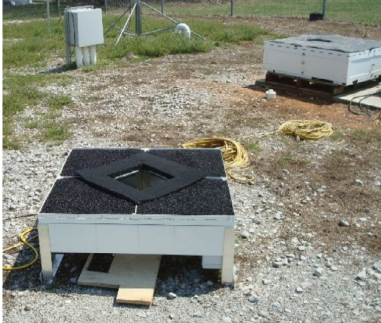
Figure 4. An example of the 2DVD (foreground—third generation compact type; background—second generation low-profile type), which is the type of disdrometer that was used to construct the weather taxonomy for rain described herein.
