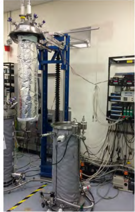
Figure 6. Cryostat-100: (a) Basic schematic and (b) overall arrangement with lift mechanism.
