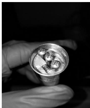
Figure 4. The Internal structure of the RDA for the thermal atomization process
