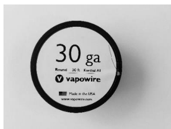
Figure 6. The Kanthal wire used to build a custom resistive coil of the RDA
