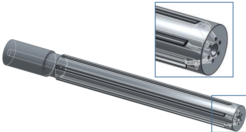
Figure 3. Ceramic insulator with propellant feed channels.
