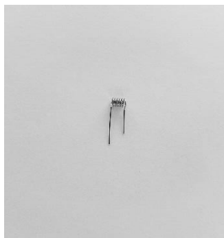
Figure 5. The conventional pre-made resistive coil for the RDA of the thermal atomization process
