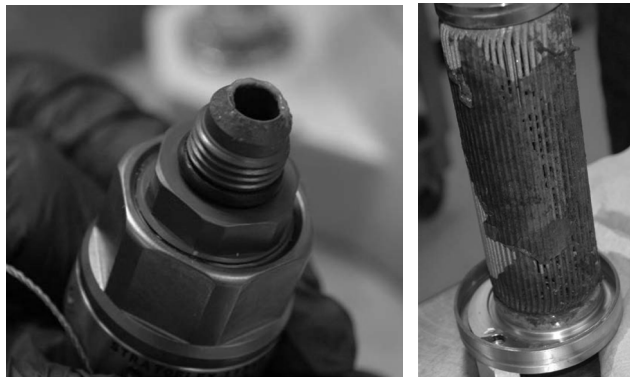
Figure 4. Biofilm on a Quick Disconnect (QD) valve and a filter from the Distillate Filter.
