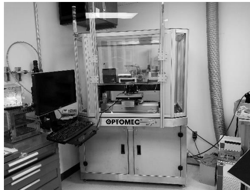
Figure 1. Optomec Aerosol Jet® printer 300 (AJ 300) Series Located at MSFC
