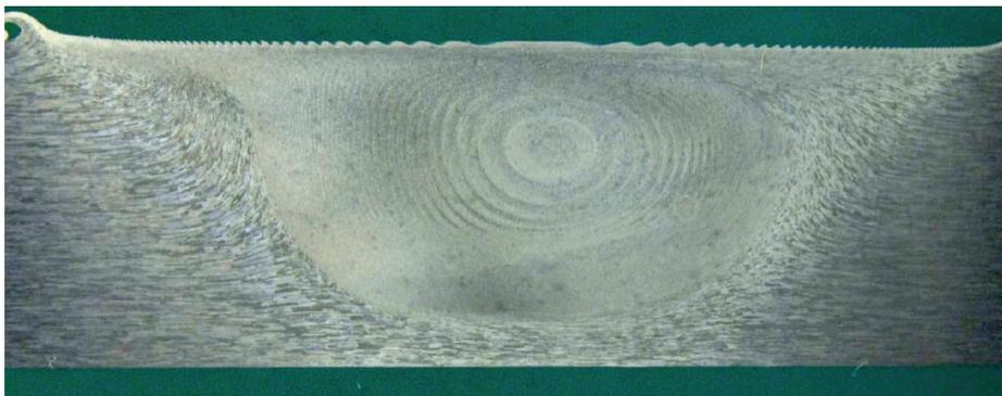
Figure 9. Transverse weld: (a) Schematic synthesis of features due to various FSW flow components on transverse weld section and (b) transverse bead-on-plate section in 0.5-in-thick, 2219 aluminum alloy (400 RPM, 2 in/min, 3° lead angle, courtesy of J.C. McClure).
