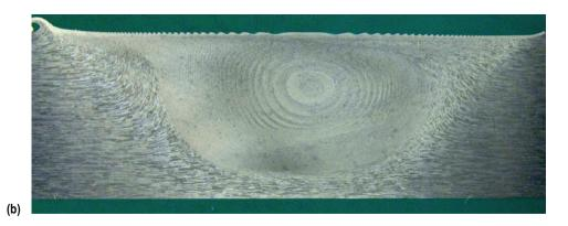
Figure 9. Transverse weld: (a) Schematic synthesis of features due to various FSW flow components on transverse weld section and (b) transverse bead-on-plate section in 0.5-in-thick, 2219 aluminum alloy (400 RPM, 2 in/min, 3° lead angle, courtesy of J.C. McClure). In table 2 the flow components are related to controlling factors within weld parameters and tool geometry.
