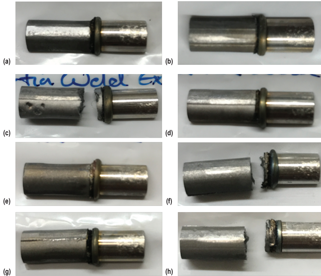
Figure 9. Images of rhenium/Inconel 718 inertia welds: (a) Sample 7, (b) sample 8, (c) sample 9, (d) sample 10, (e) sample 11, (f) sample 12, (g) sample 13, and (h) sample 14.
