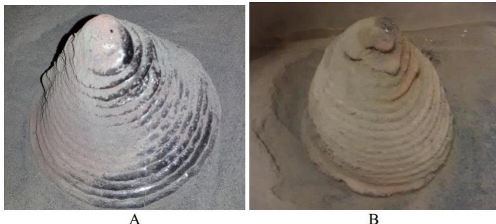
Bench-top scale freestanding structures created by Swamp Works 3D Regolith Construction process: A) BP-1 Hollow Cone Structure; (source:...
