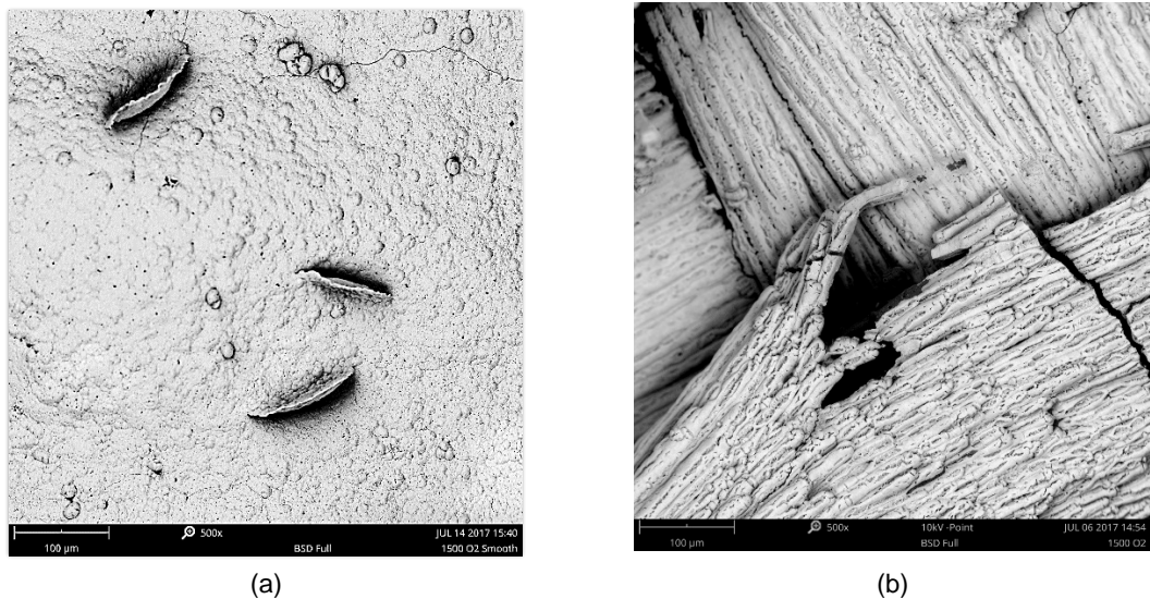
Figure 5.—Scanning Electron Microscope (SEM) images of a 1500 °C oxidation tested specimen. Image (a) shows the “smooth” side of the sample tested at 1500 °C for 100 hr, while image (b) shows the “rough” side of the same sample. One can note the difference in grain texture, as well as the beginnings of spallation on the “smooth” side.
