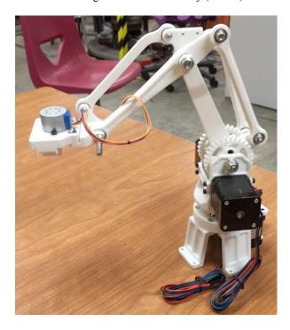
The uArm Swift robot arm was acquired as an open-source, Arduino-based alternative to the DoBot Magician. While less precise than the DoBot Magician due to its servo motor drive system, the uArm Swift provided an open-source alternative to the DoBot. We were able to successfully develop software limitations
