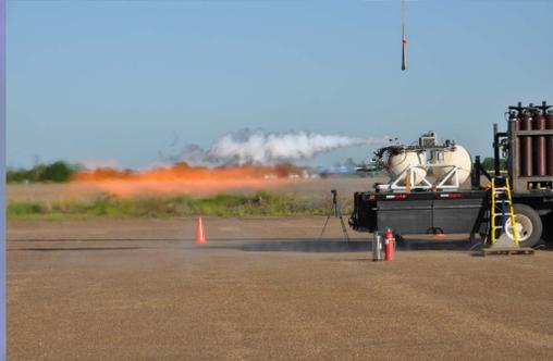
Specific impulse is the measure of efficiency for rocket propulsion, similar to miles per gallon for a car. The unit of measure for specific impulse is seconds, [s]. Specific impulse is the change in momentum per unit of propellant. A bipropellant rocket motor with a high specific impulse can provide more change in momentum than a different motor with a lower specific impulse; using the same amount of propellant.
