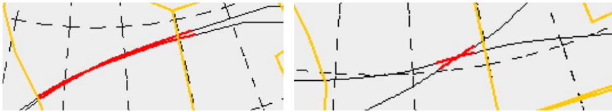
Figure 22. Examples of a “continuous conflict” (left) between trajectories from Brussels (EBBR) to New York, Liberty (KEWR) and from Frankfurt (EDDF) to Charlotte (KCLT); and a “spot conflict” (right) between trajectories from New York, Liberty (KEWR) to Oslo (ENGM) and from Chicago, O’Hare (KORD) to Rome (LIRF).
