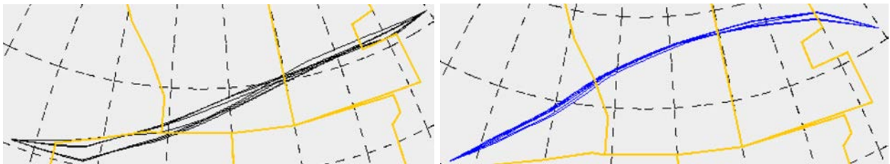
Figure 9. Trajectories between London, Heathrow (EGLL) and New York, J.F. Kennedy (KJFK); 13 eastbound flights (left, black) computed with wind forecast at 0000 UTC distributed between 4 FLs (FL330, FL350, FL360, and FL370); and 9 westbound flights (right, blue) computed with wind forecast at 1200 UTC distributed between 6 FLs (FL320, FL340, FL350, FL360, FL370, and FL380)
