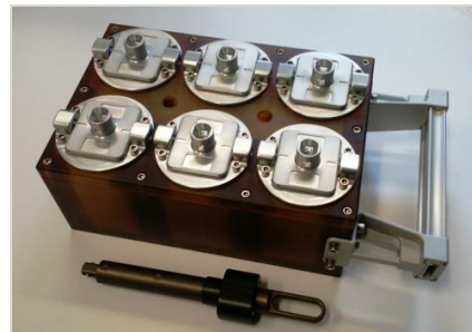
Prototype EVA Swab Kit 8-Sample Caddy (6 on one side, 2 on reverse side - not shown) and Tool Handle
