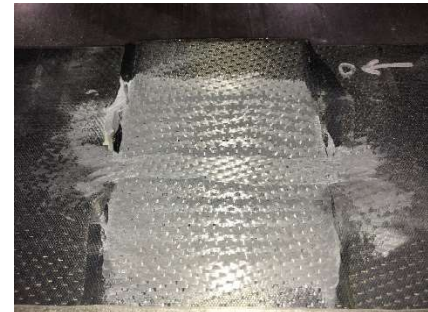
Figure 5. Tapered Scarfing on Test Panel Doubler
