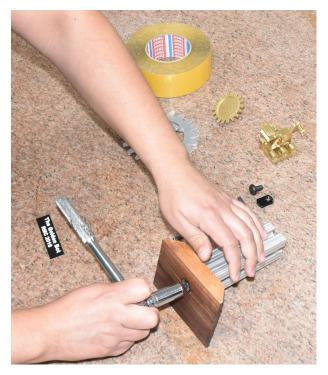
Great care is needed in this step. The gear will be balancing in your hand and if dropped it could impact the wood leaving a dent. Pass the 5/16-18 x .687" (part# 3330) bolt through the gear's bolt hole and into the T-nut (part # 3278).
