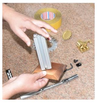
Finishing attaching the column to the base by placing the base and column as shown. By having the edge of the base and the column lie flat on the surface, they will be parallel to each other. Tighten the bolt while avoiding splitting the wood.
