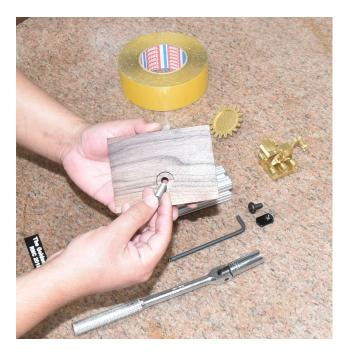
Start screwing the column's tapped hole to the exposed bolt. Be careful to avoid scratching the wood.
