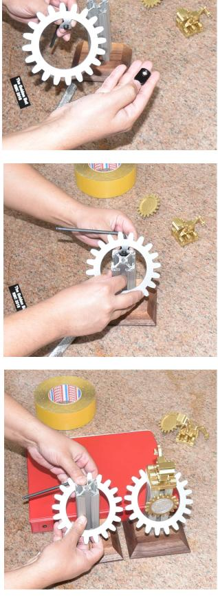
Next, slide the coin holder into place. Depending on the spray paint, there may be resistance. Either sand paper or an X-acto blade to scrape away the paint.
